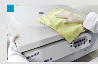
Switch off centrifuge and wipe centrifuge housing. If required, clean with mild detergents.
