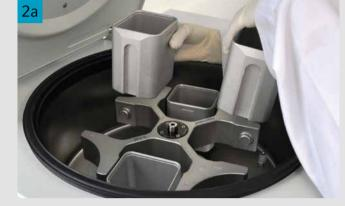
Remove buckets and rotor. For refrigerated centrifuges: > Defrost the ice on the rotor chamber surface. > Empty and clean the water collection tray.
