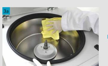
Wipe rotor chamber and motor shaft. If needed, wipe with mild neutral detergent or use 70 % alcohol for disinfection.
