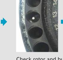
Check rotor and buckets for corrosion. Take out of service if corroded or if any sign of damage is detected.
