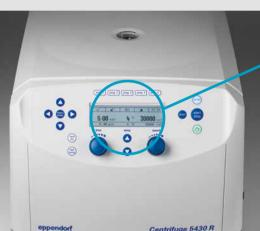
Error 15 Load rotor symmetr., check load ever Press OPEN, repeat run. 30:00 min
