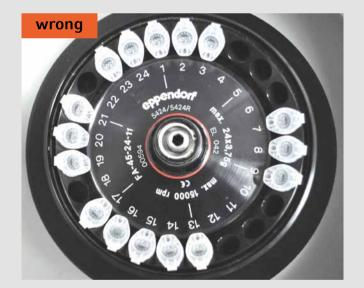
Fixed-angle rotors: Load symmetrically and balance weights.
