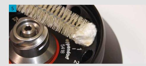
If needed, autoclave rotor, rotor lids and buckets at 121 °C, 20 min. (Never use UV, beta, gamma radiation, or any highenergy radiation source.) Clean rotor, rotor lid, rubber seal, buckets, and adapters with damp lint free cloth and diluted detergents, alcohol, or alcohol containing detergents. Afterwards, wipe seals with wet cloth and rinse thoroughly with distilled water. Use test-tube brush with non-metallic tip to clean the rotor bores.
